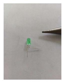
Snip a little off the bend lead to allow the LED to be closer to the Expansion board.
