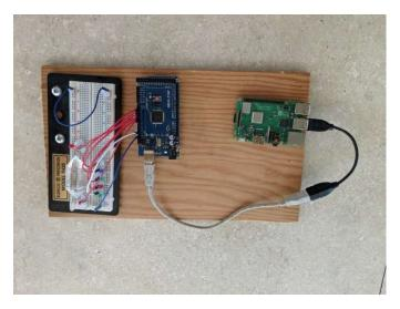
Photo of my first AetherOne system running on a Raspberry Pi 3B+ with a Mega Arduino board. The LEDs are broken out onto a breadboard with jumper wires between the Mega and the LEDs.
